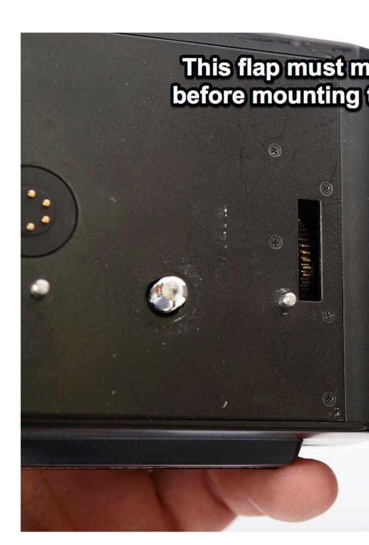
Before mounting the winder on the bottom of the camera, first open the flap on the bottom of the camera, as shown in the image above.
