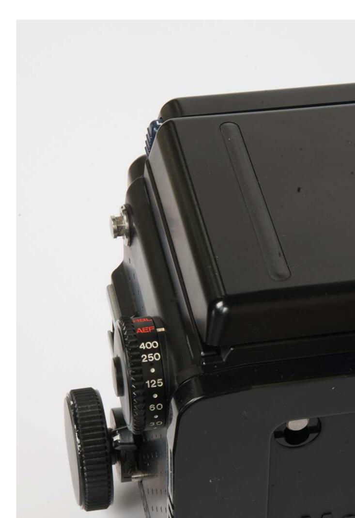
The front cap is easy to install (like a lens), but it does not lock very well. For the back cover, set the RM lever in the R position to install it or to remove it, and back in the middle place in the meantime to block it. Unfortunately, Mamiya has not made any cover to replace the viewfinder, but I think it's essential to send the focusing screen you use for the repairs.
