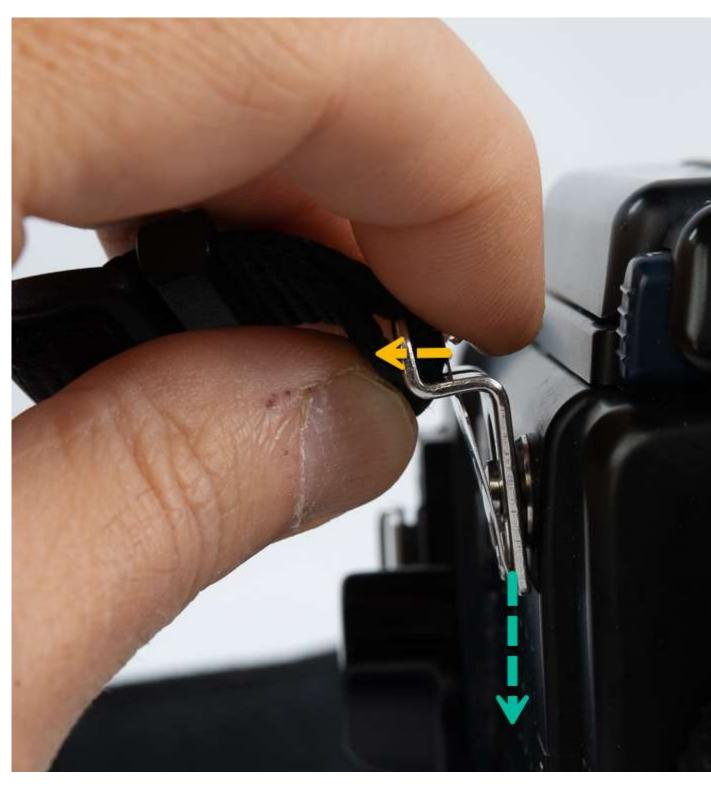
Pull out the thin metal part as shown in the picture and pull the clip assembly downwards.
