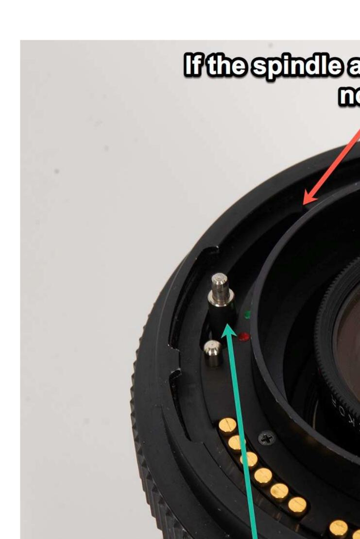
The two spindles must be in between the red and green dots on the rear of the lens. If not, try to lightly push them with your fingers until they move to the position they have to be. When set to the correct position, the shutter will be open.
