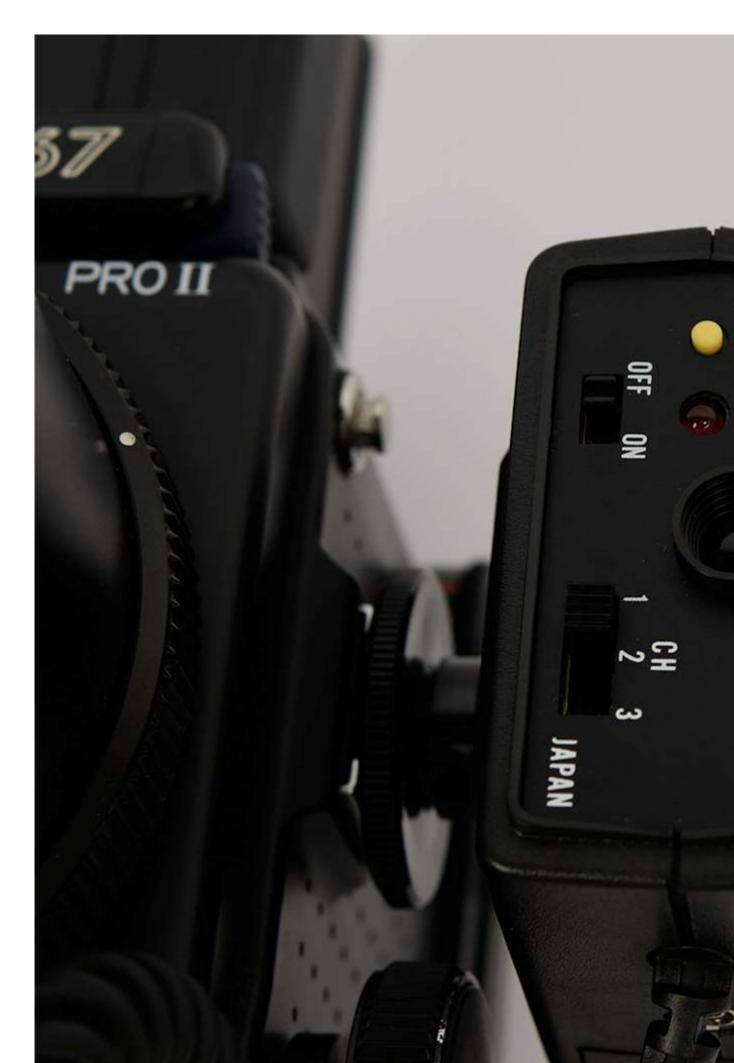
You have three different channels (frequencies) available. Be mindful to always set the same channel on both the remote and receiver. The transmitter needs 2x R6/AAA batteries, and the receiver needs a 1x 9V0006P (or HN22, NR22, 6LR61...) battery.
