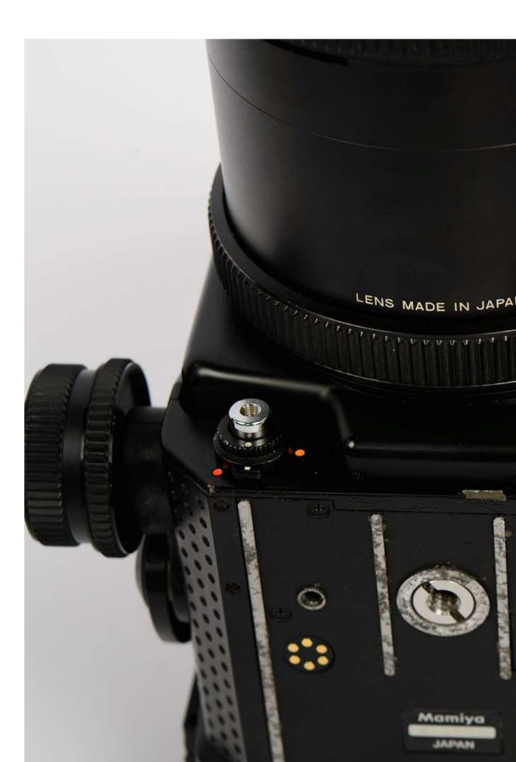
You can lock the plug on the camera: it's the "L" position.
