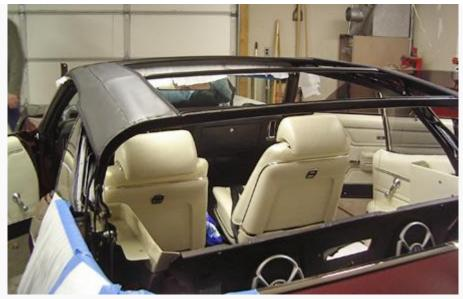
Some cars have two stay pads, one on each side, from the header to the rear bow. In some cars, there are four (two front and two rear, or quarter, pads.)
