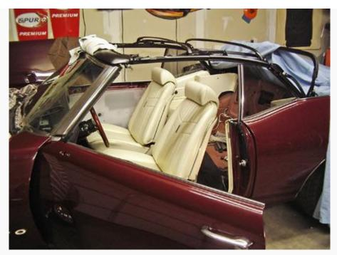
This top frame was cleaned, painted and rebuilt. Reproductions of the chrome plated top latches for this top were available.
