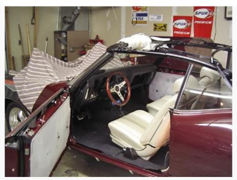
You will have to check the fit of the side glass against the rebuilt top frame to avoid breaking the glass when the side window is raised.
