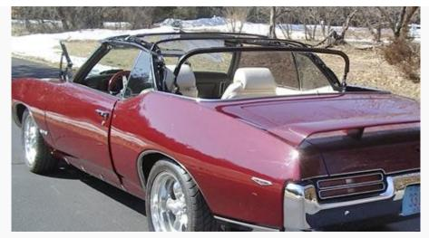
For proper geometry use spacer sticks between bows or take a bow height measurement from center of top frame to center of the rear body tub.
