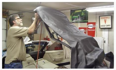
An installer uses an air stapler and stainless steel staples to attach the front of the new convertible top to the header bar.
