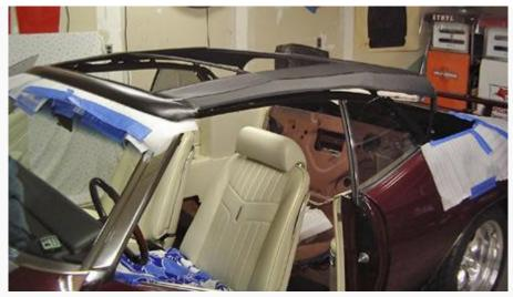
The term top pad or stay pad refers to the covered foam or the padded webbing that runs under the top and along the edges of the top frame.
