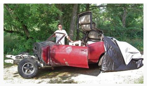
This car has a good top frame, but it has rivets that need replacement, the bows need refinishing and the fabric top is badly in need of replacement.
