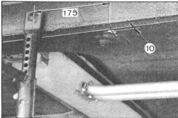
3°) Drill hole  $\phi$  10 mm under each rear floor panel.
