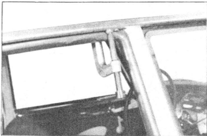
Tighten alternately at left and right-hand side working towards the rear.
