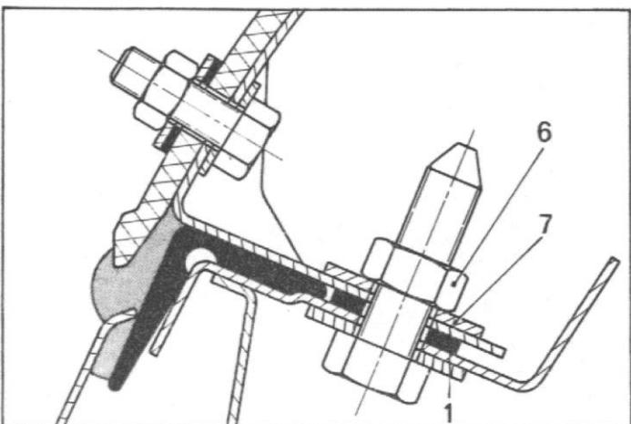
12. Position roof fixing screws in line with centre pillars and rear window panelling.
