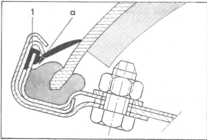
28. Using a putty knife, free the « SOLBIT » strip from the edge of siderail at « a » to allow clearance of heel of rubber moulding (1).
