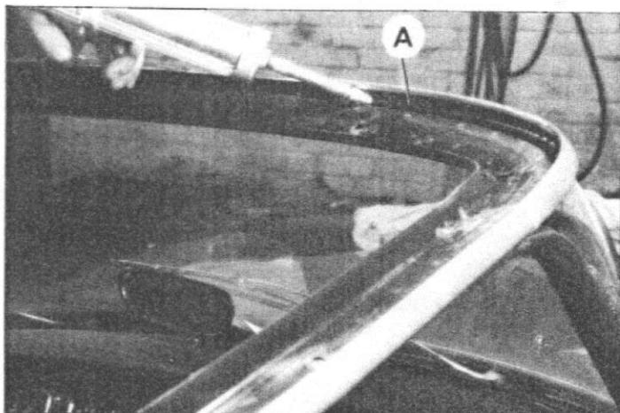
Using a jet gun, eject a continuous ribbon of sealer ( PLASTIJET type ) around the front part of the roof siderail.
