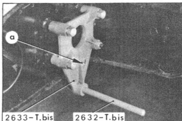
**IMPORTANT NOTE :** At the foundry, certain fixtures are stamped at point « a » : « before April 1958 » on one side and « after April 1958 » on the other side. The side which should be applied to the front bosses is that which corresponds to the introduction date of the vehicle. On the side marked « before April 1958 » there is a difference of 2 mm between the location of the upper and lower bosses; on the side marked « from April 1958 » all four bosses are evenly spaced.
