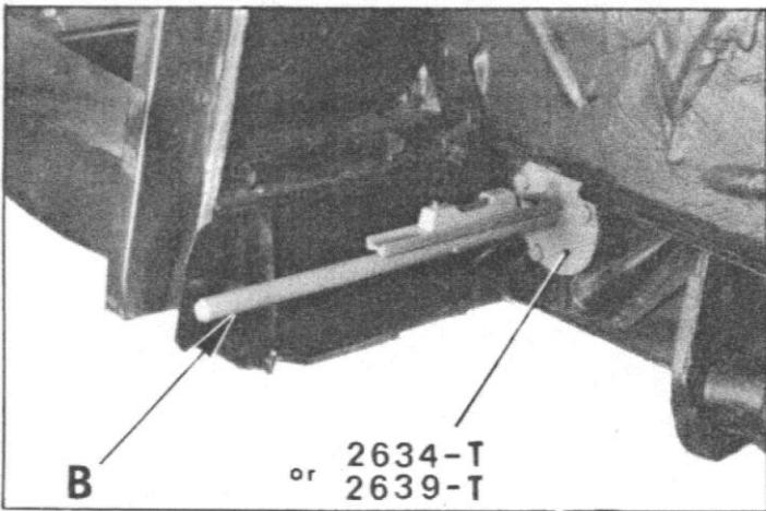
Place the adjusted spirit level on the rear rod ( B ) the difference as indicated by the level must not exceed 3.5 mm per meter.
