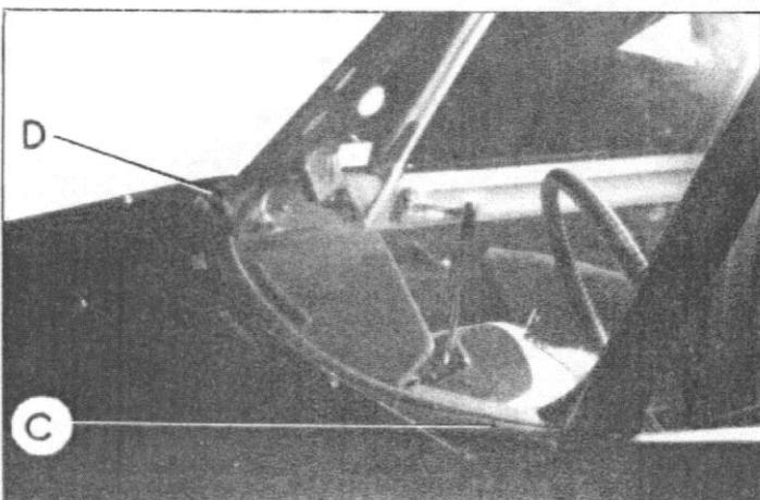
Compress sealing compound well down into lower corners of windscreen.
