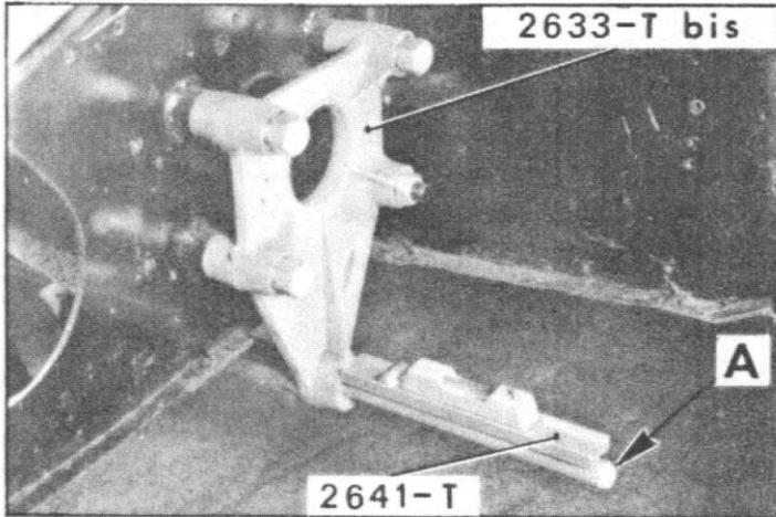
c) **Checking distortion of front and rear section :**
