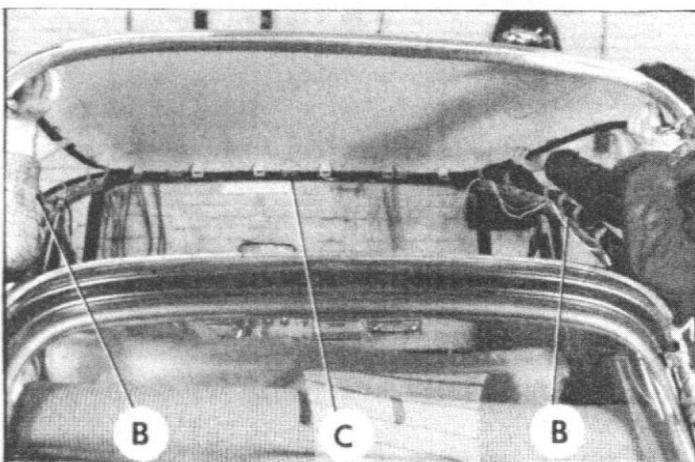
Position the fourteen remaining screws ( use washers under screwheads ). Fit nuts but do not tighten.
