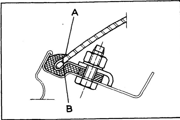
1°) Remove band of sealing putty around front of roof,
