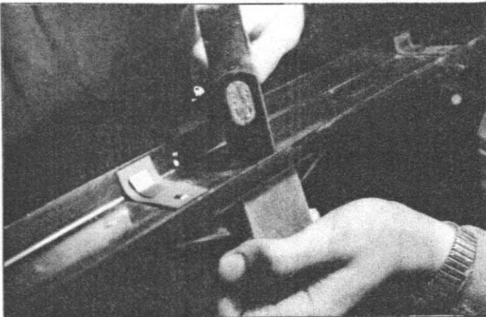
NOTE : Should it be necessary to straighten the roof fixing lugs, care must be exercised to avoid deformation to roof crimping.
