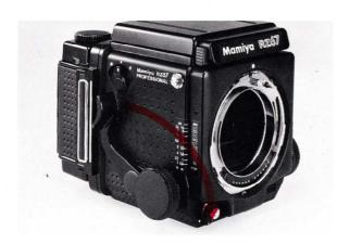
**1.** Set the mirror of the camera body by sliding the cocking lever all the way toward the front of the body.
